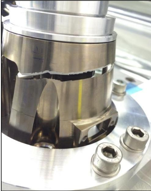
Figure 6. Ultimate shear load of EM-1bracket: 20kN!
