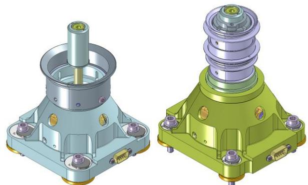
Figure 2. NELS application variants: Left: Antenna HDRS, Right: Solar Array HDRS
