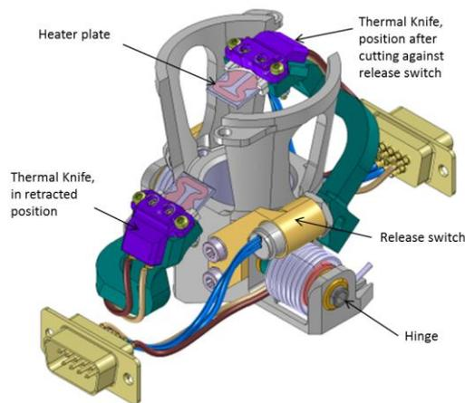
Figure 4. Thermal Knife assembly (EM-2)
