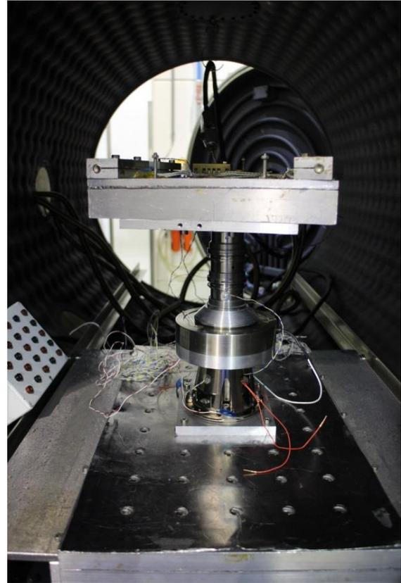
Figure 7. NELS stack in vacuum chamber for thermal cycle test. Top and bottom cooling and heating establish a thermal gradient in the stack
