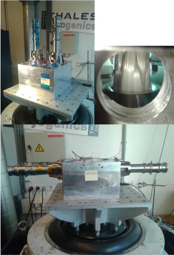
Figure 9. Stacks on vibration table at Thales. View on cutting area of restraint cable after vibration testing.
