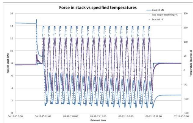
Figure 8. Temperature and pretension during 20 cycles.
