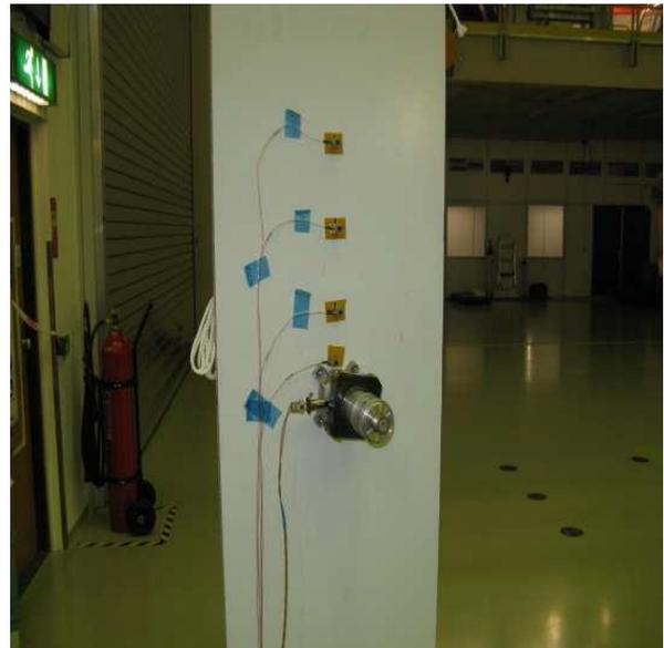
Figure 10. NELS hold down mounted on free hanging sandwich panel. Accelerometers placed 100mm interspace
