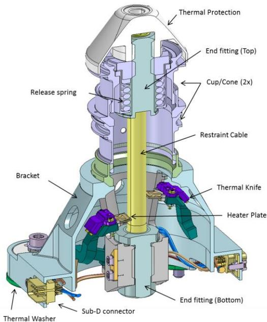
Figure 3. Cross section of NELS (EM-2)
