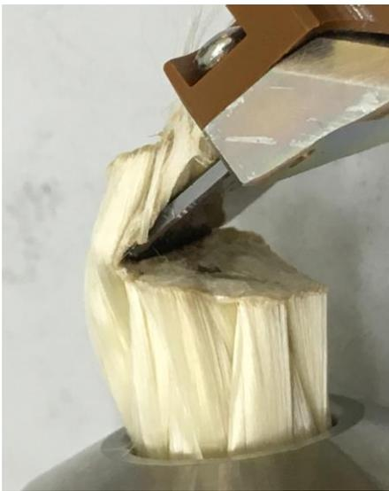
Figure 5. Thermal Knife cutting Vectran cable
