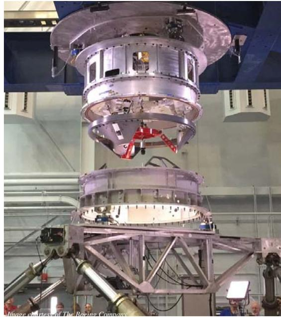
Figure 10. Flight Configuration SCS in 6DOF Test
