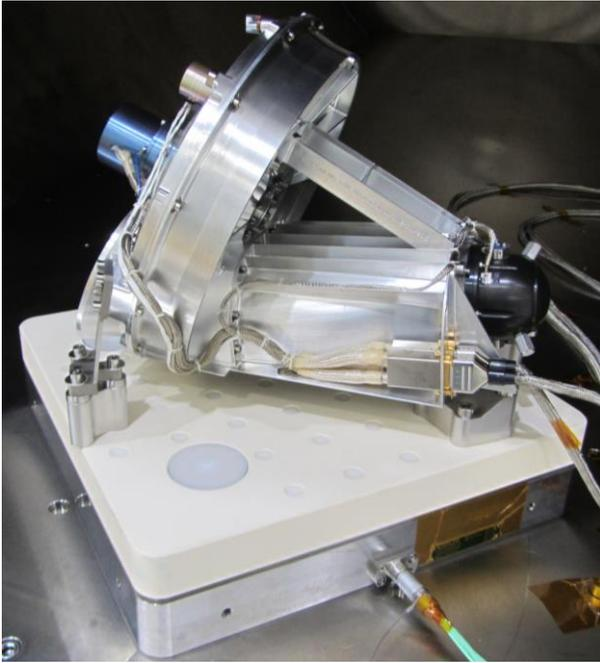
Figure 10. UVN CAA mounted on  $\mu$ Vib table
