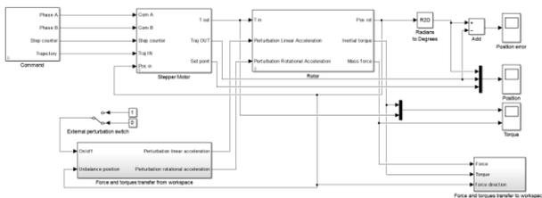
Figure 9. Micro-vibrations Simulink model
