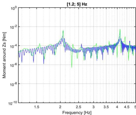
Figure 11. Simulated (blue) vs measured (green)  $\mu$ Vib
