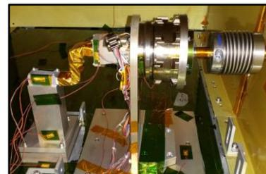
Figure 14. Flexible thermal strap
