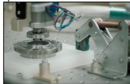
Figure 9. Wave generator assembly insertion in flex cup
