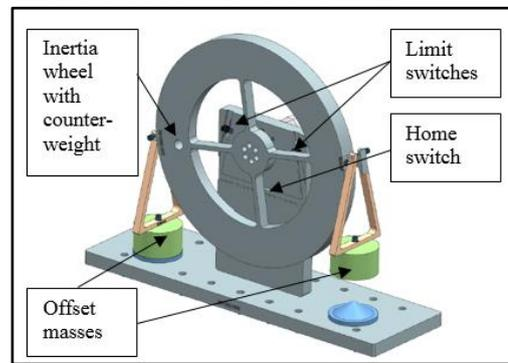
Figure 18. Inertia wheel test vehicle
