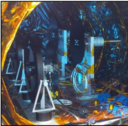
Figure 16. Both life test vehicles in TVAC
