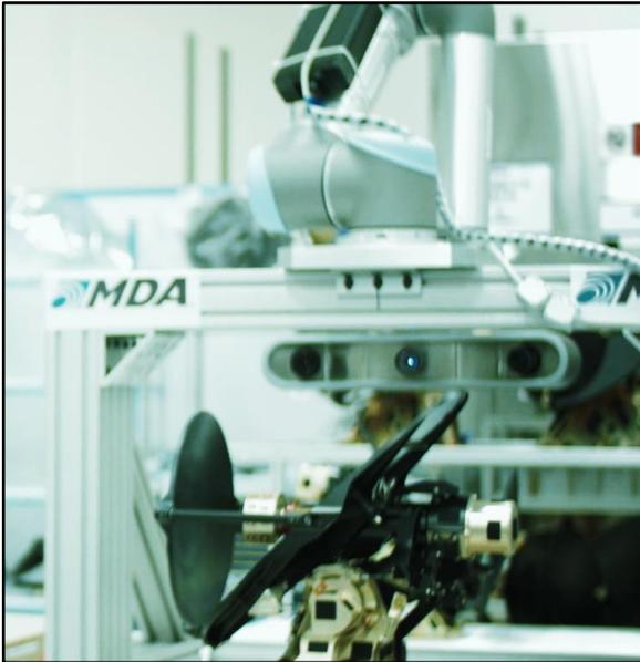
Figure 10. Photogrammetry robot
