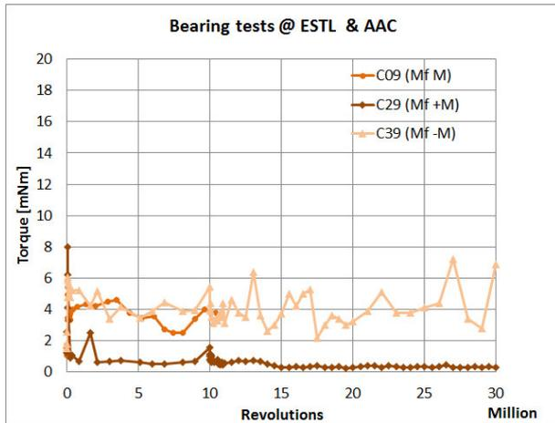
*Figure 7: Ball bearing tests in high vacuum on mineral fibre based composites: C29 with higher MoS<sub>2</sub> shows definitely the lowest torque. (Tests until 10mio rev done at ESTL)*
