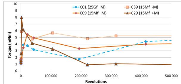
**Figure 5:** Ball bearing tests: torque in high vacuum (detail showing start) [4]
