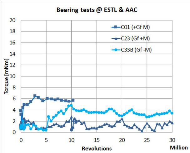
*Figure 8: Ball bearing tests in high vacuum: on glass fibres based composites: C23 with higher MoS<sub>2</sub> shows low torque, but more noise. (Test of C01 done at ESTL.)*
