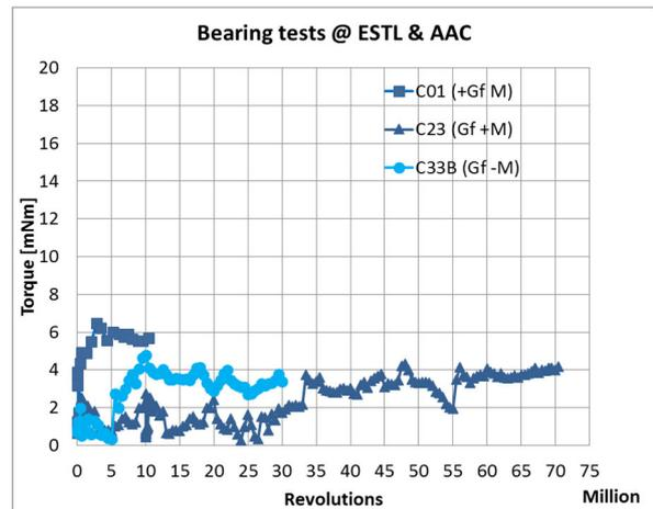
*Figure 9: Ball bearing tests in high vacuum: on glass fibres based composites: C23 with higher MoS<sub>2</sub> shows later an increase of torque. (Test of C01 done at ESTL.)*
