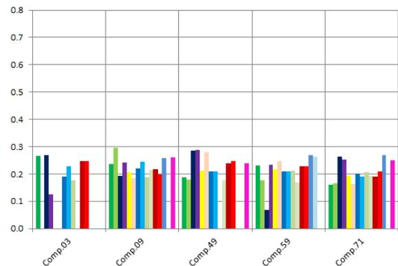
Figure 3: Friction coefficient for new composites based on European mineral fillers (C49, C59) and aramid fibres (C71) compared to US based mineral fibres (C09) and glass fibres (C03): Friction in all test cases in range 0,18-0,30.
