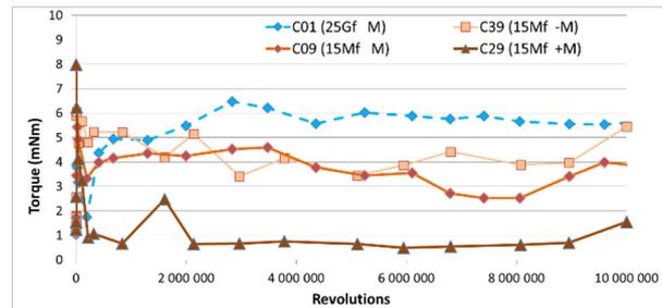
**Figure 6:** Ball bearing tests: torque in high vacuum (full test duration), C29 with higher MoS<sub>2</sub> shows definitely lowest torque. [4]
