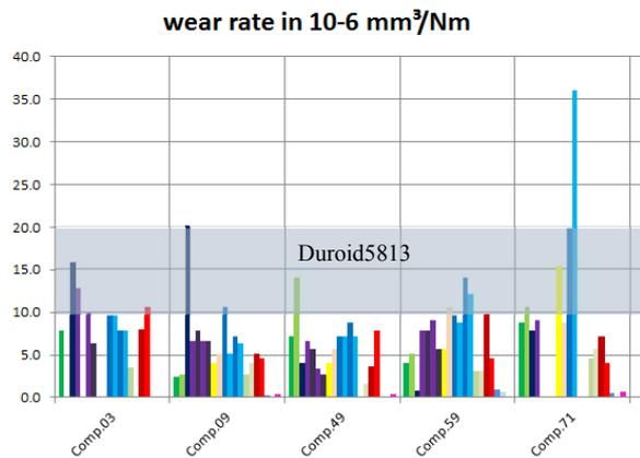
**Figure 4:** Wear rates for new composites based on European mineral fillers (C49, C59) and aramid fibres (C71) compared to US based mineral fibres (C09) and glass fibres (C03).
