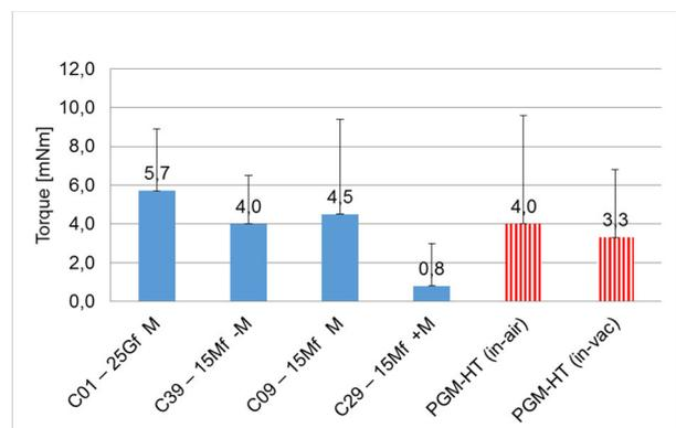
*Figure 1: Ball bearing tests: torque in high vacuum, compared to literature (for PGM-HT) [4]*
