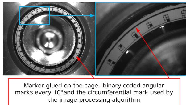
Marker glued on the cage: binary coded angular marks every 10° and the circumferential mark used by the image processing algorithm
