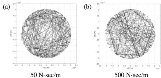
Figure 23: Trajectory for the increased damping coefficient (b)
