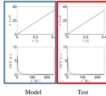
Figure 17:  $\alpha(t)$  from the model (left) and the test (right)
