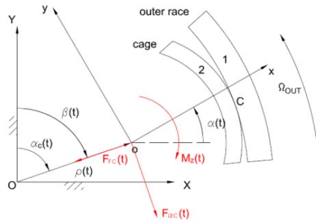
Figure 2: Contact cage / outer race
