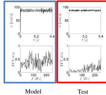
Figure 18:  $\dot{\alpha}(t)$  from the model (left) and the test (right)
