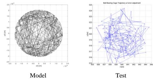
Figure 19: Cage trajectory from the model (left) and the test (right)
