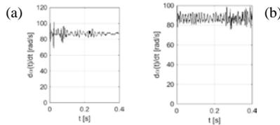
Figure 22: Numerical simulation results with 500N·sec/m damping at cage races (a) and 50 N·sec/m at cage races (b)
