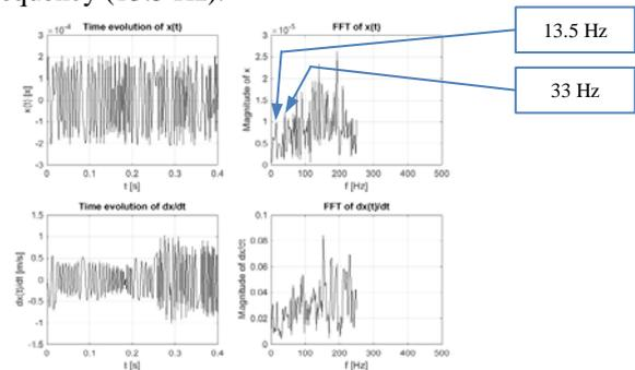
Figure 20: Main frequencies – shaft and cage (model)
