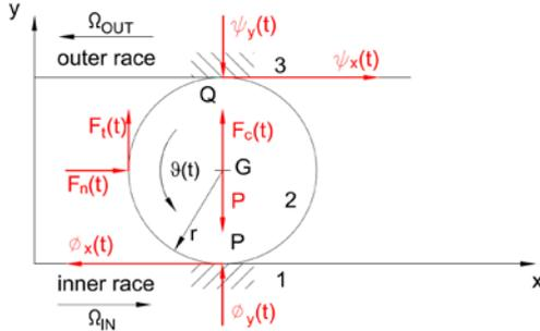
Figure 5: Forces acting on the balls
