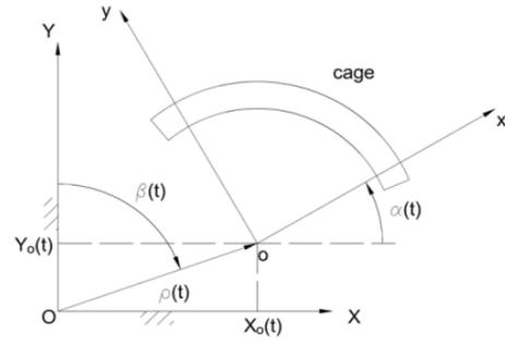
Figure 1: Motion of the cage – reference axes
