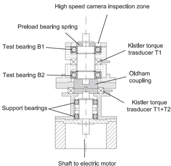
Figure 8: Ball bearing test bench at ESTL
