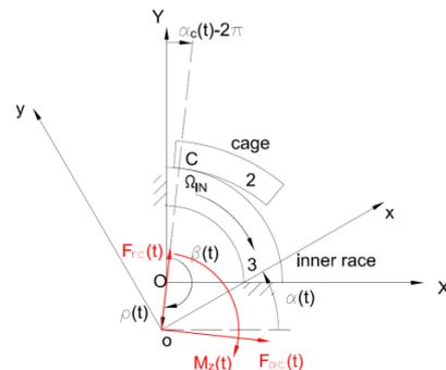
Figure 3: Contact cage / inner race
