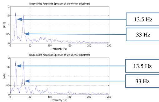
Figure 21: Main frequencies – shaft and cage (test)
