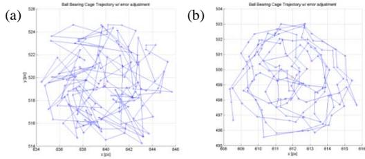
Figure 15: Cage's trajectory: (a) unlubricated, (b) lubricated
