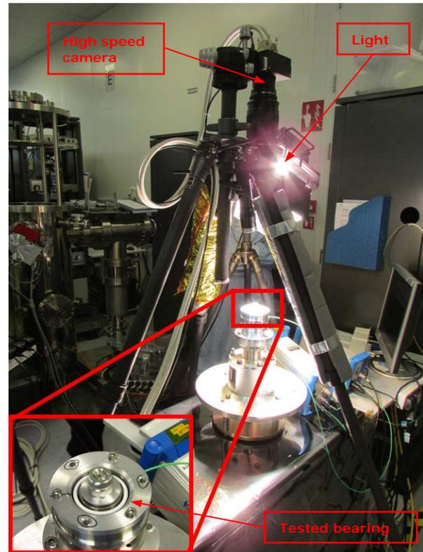
Figure 9: ESA High Speed Camera test stand configuration
