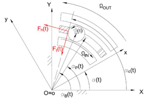
Figure 4: Contact cage/ balls
