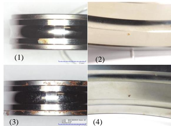
Figure 18 : (1, 3) state after 6h and 48h of test on ring with non-optimized treatment and (2,4) ) state after 6h and 48h of test on ring with optimized treatment.
