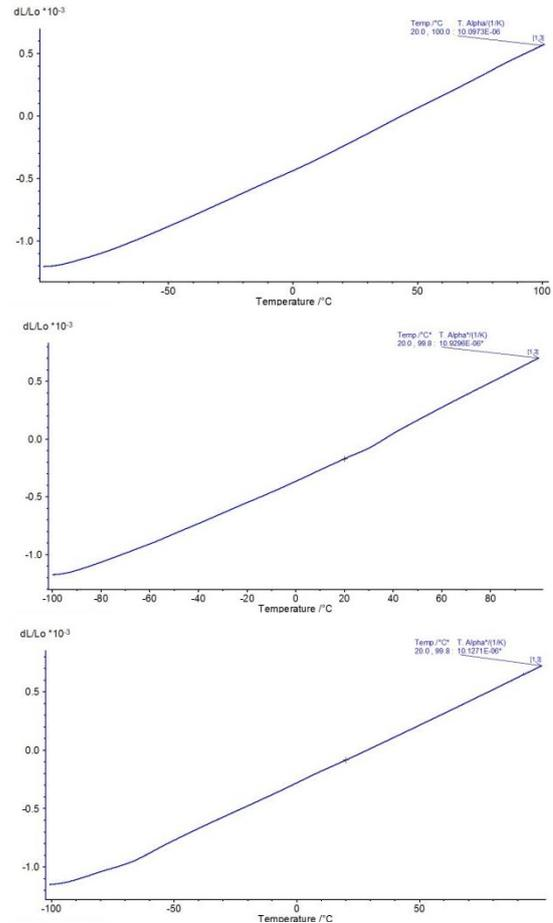
Figure 6: Expansion depending on temperature
