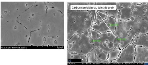
Figure 16: Differences of microstructure of XD15NW obtain (1) with the optimized thermal process and (2) SCC specimens thermal process
