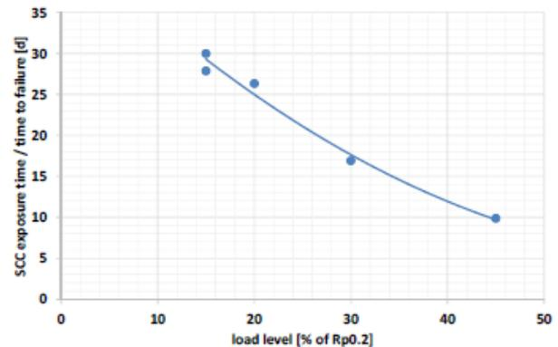
Figure 14: SCC exposure time VS load level
