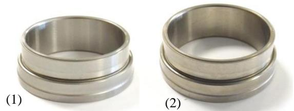
Figure 17: (1) Initial state of specimen, (2) state of specimen after 48 h of high humidity test.
