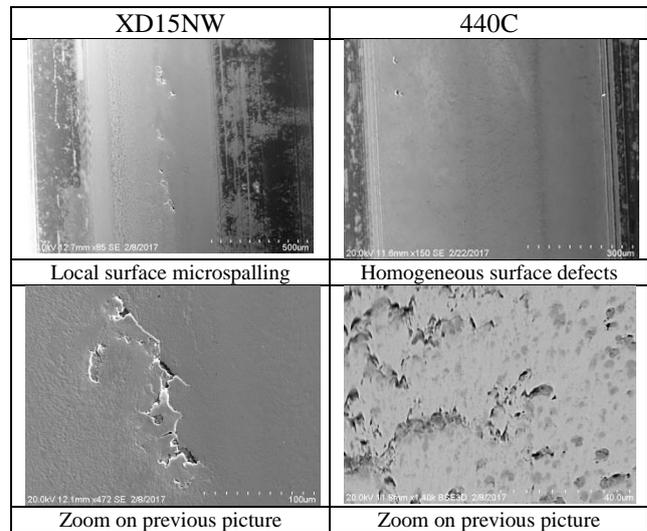
Figure 10: Post-test SEM inspection on XD15NW and 440C rings
