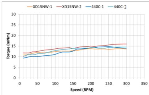
Figure 9 : Torque vs Speed measurement @test temperature
