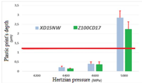
Figure 5: Plastic print's depth depending on Hertzian pressure
