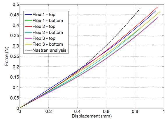
Figure 12. Comparison of the force/displacement behaviour between 3 different flexures (top and bottom side of each one) and the analytical data obtained with nonlinear analysis in Nastran
