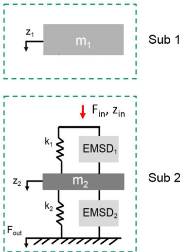
Figure 9. Separation of the 2-collinear-DoF system into two subsystems
