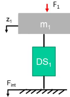
Figure 10. Representation of the subsystem 1 that is connected to the equivalent dynamic stiffness produced by the subsystem 2
