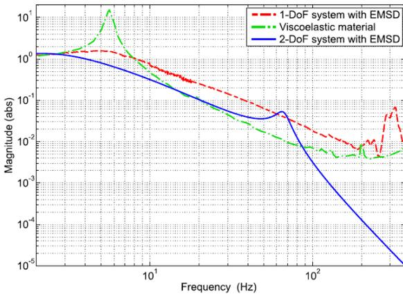
Figure 4. Comparison of the force transfer functions between three different damping systems: 1-DoF system with EMSD presented in [5], viscoelastic-material passive isolator presented in [1], and the 2-collinear-DoF system proposed in this paper
