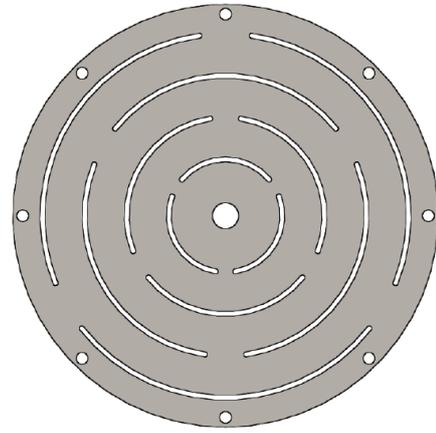
Figure 5. Flexure design finally chosen for the strut
