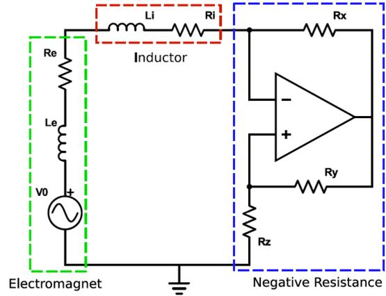
Figure 2. Schematic of the EMSD electric circuit used for the 2-collinear-DoF system. The shunt circuit includes the negative resistance converter and an iron-core inductor
