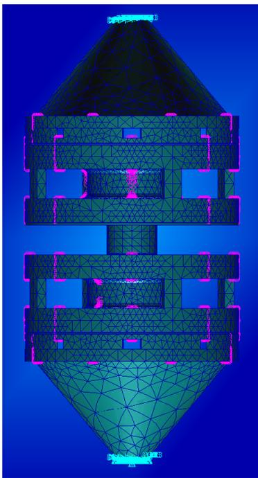
Figure 7. Patran model of the 2-collinear-DoF strut prototype
