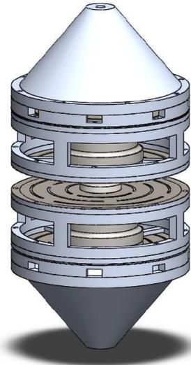
Figure 6. Preliminary design of the 2-collinear-DoF strut prototype.
