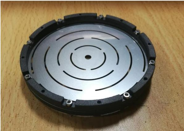
Figure 11. Support used to measure the axial stiffness through a compression/tension machine
