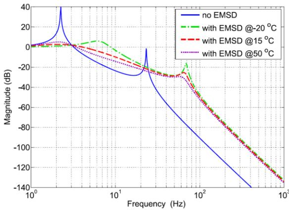
Figure 3. Comparison of the analytical solution of the force TFs between the system without EMSD (i.e. electromagnets in open-circuit conditions) and the system with EMSD at three different temperatures.
