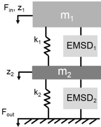
Figure 1. Schematic representation of the 2-collinear-DoF model
