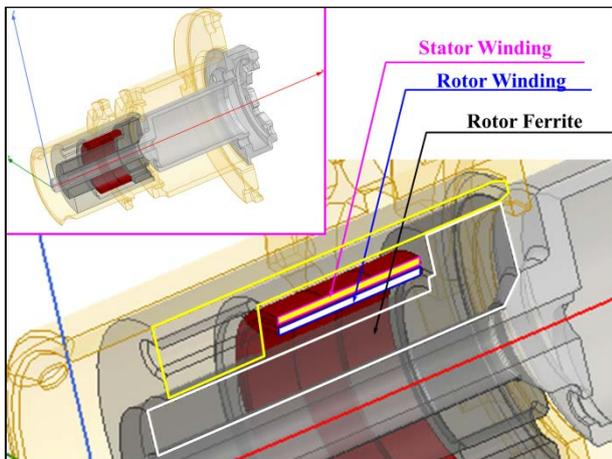
Figure 7: Magnetic part geometry
