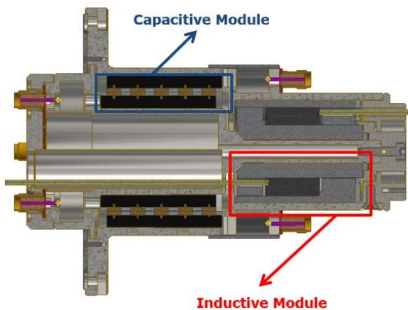
Figure 4 : Cross Section of the demonstrator
