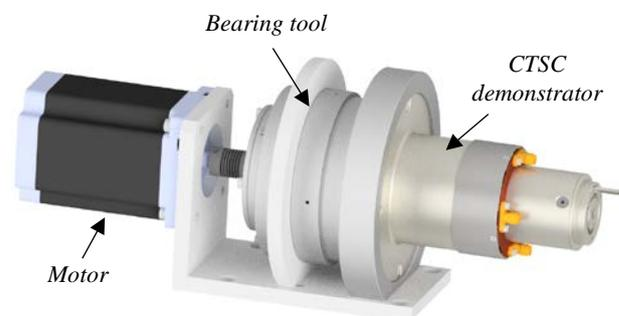
Figure 3 : demonstrator with bearing tool and motor
