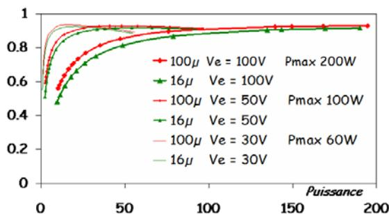
Figure 2: CNES prototype power transmission efficiency
