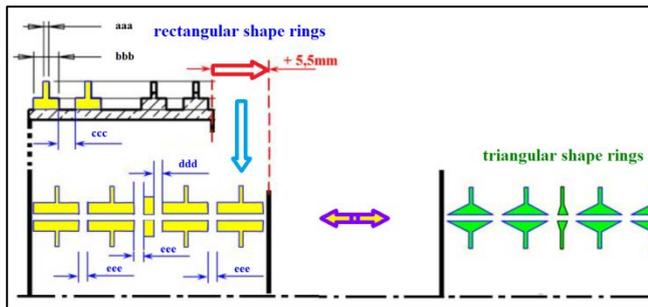
Figure 9 : Example of the different geometrical parameters changes used in calculations
