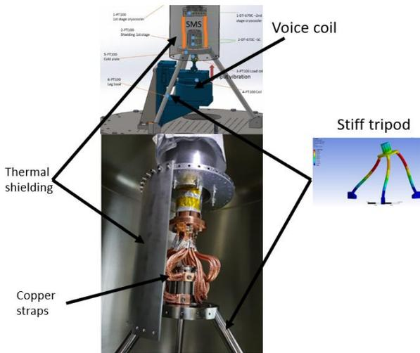
Figure 4: Test bench for axial characterization at 15 K
