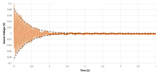
Figure 8: Displacement vs time of the suspended mass. It is observed that after a sudden event the system is stabilized in its equilibrium position.
