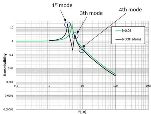
Figure 1: Expected transmissibility curve of the vibration's isolator for a 12 kg FPA
