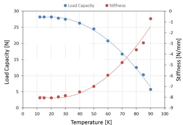
Figure 6: Axial load capacity and stiffness vs. temperature. Red dots- Stiffness variation vs. temperature. Blue dots- Force variation vs. temperature.
