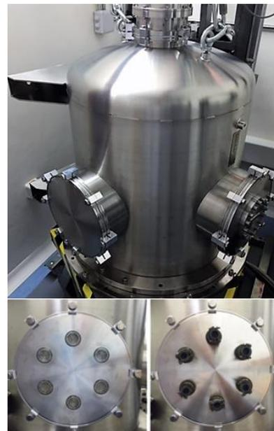
Figure 3: High Vacuum Chamber with 4 K Cryohead
