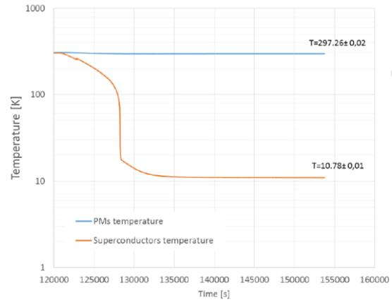
Figure 2: Thermal disconnect feature (zero thermal conductivity)
