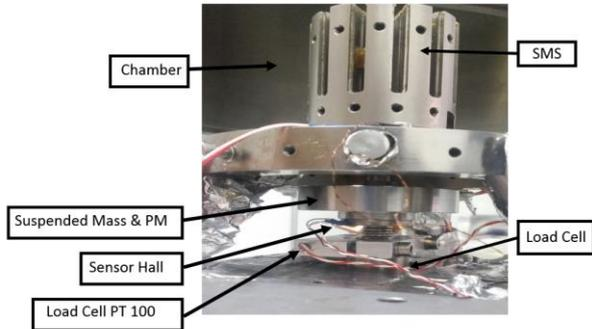
Figure 7: Free oscillation test for damping ratio characterization.
