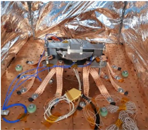
Figure 8 Test article and test set-up installed on cryostat baseplate
