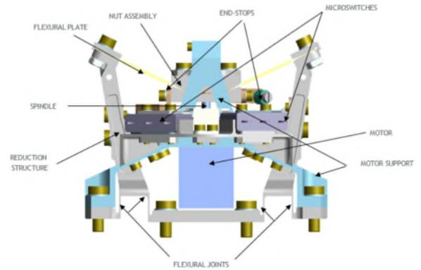
Figure 2 Actuator main parts
