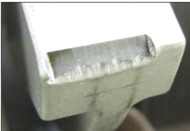
Figure 5. Hinge latch cam track after damage
