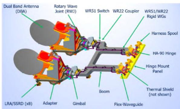
Figure 1. Antenna Wing Assembly components
