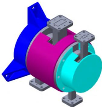
Figure 4. Solid model of the Rotary Waveguide Joint
