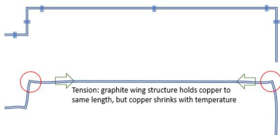
Figure 7. Thermal loads on waveguide
