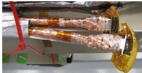
Figure 6. Copper wrapping made the harness very stiff
