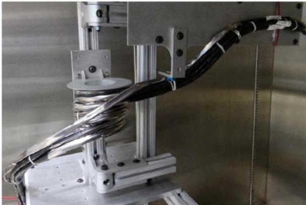
Figure 3. Hinge harness life test set up
