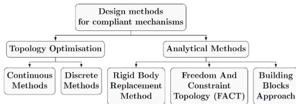
Figure 3. Different methods of designing compliant mechanisms.
