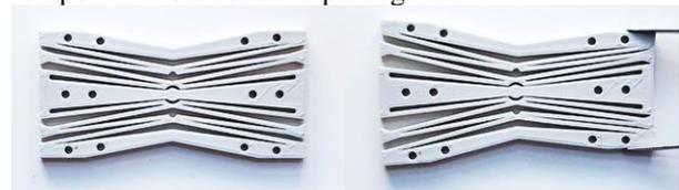
Figure 2. Compliant butterfly hinge.
