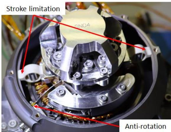
Figure 10: Anti-rotation feature for launch phase
