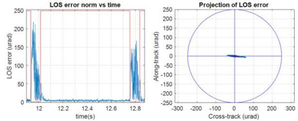
Figure 14: Pointing performance measurement on SCM-EM in time (left) and space (right) domains
