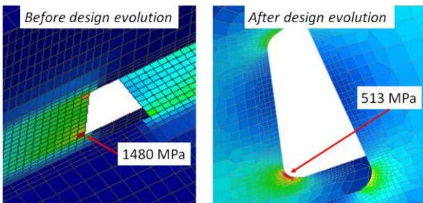
Figure 16: Finite elements analysis of the pivot before and after design modification
