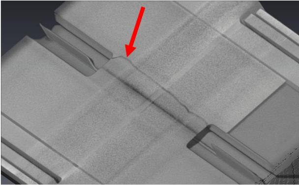
Figure 15: Micro-tomography inspection of the damaged flexural pivot
