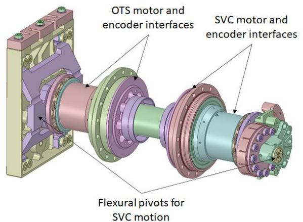
Figure 7: Internal view of the scan mechanism design
