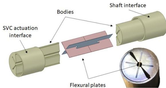
Figure 9: Overview of the flexural pivot
