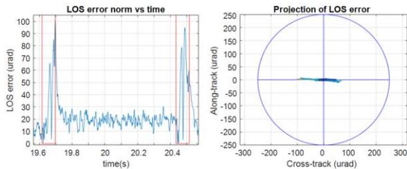
Figure 12: Pointing performance simulation in time (left) and space (right) domains (typical, BOL case)
