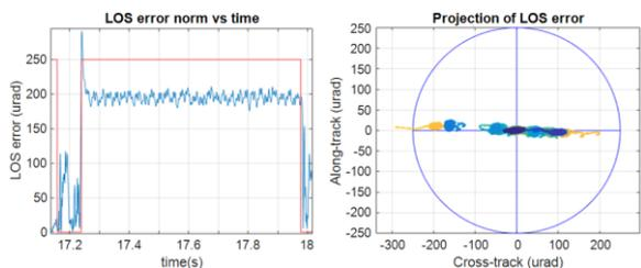
Figure 13: Pointing performance simulation in time (left) and space (right) domains (worst case EOL)
