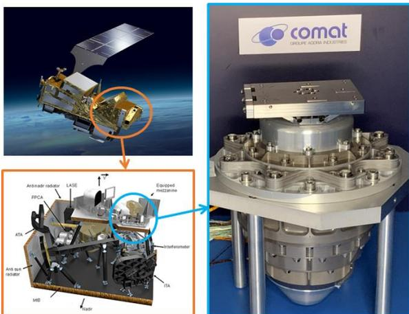
Figure 1: Scan mechanism (SCM) location on IASI-NG instrument and on MetOp-SG satellite (courtesy of EUMETSAT and Airbus DS)
