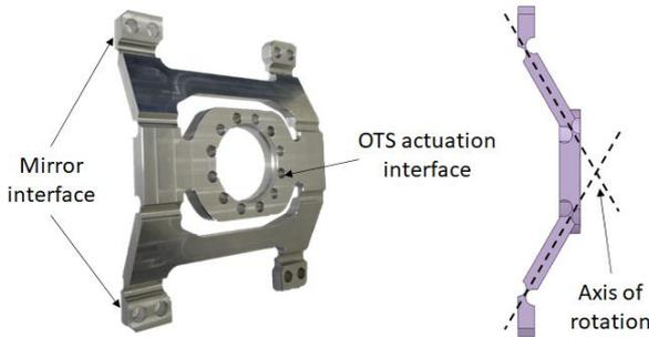
Figure 8: Overview of the RCC hinge
