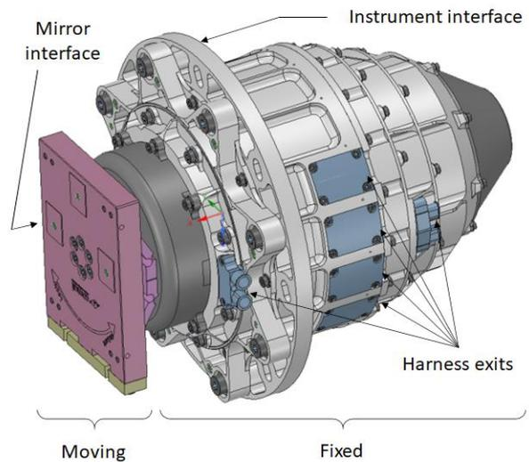
Figure 6: External view of the scan mechanism design
