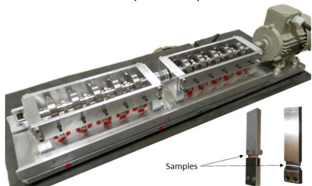
Figure 11: Breadboard for life test validation of compliant components
