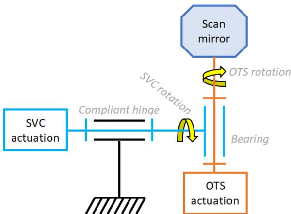
Figure 5: Kinematic principle of the series architecture
