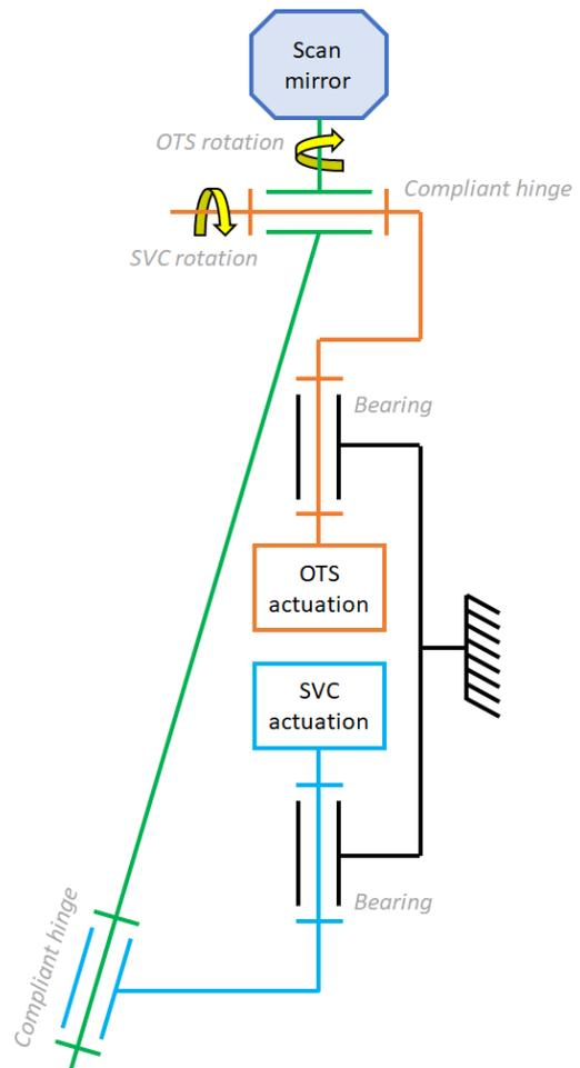
Figure 3: Kinematic principle of the parallel architecture
