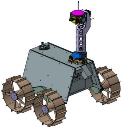
Figure 3. MAG installed in the rover. Deployed position
