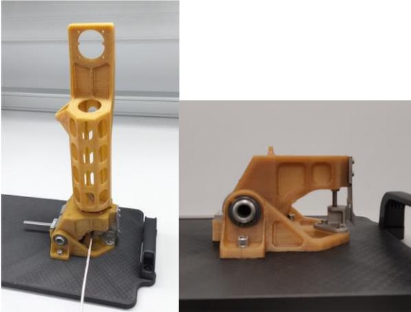
Figure 10. ULTEM 1010 parts. Mast & deployment hinge assy.
