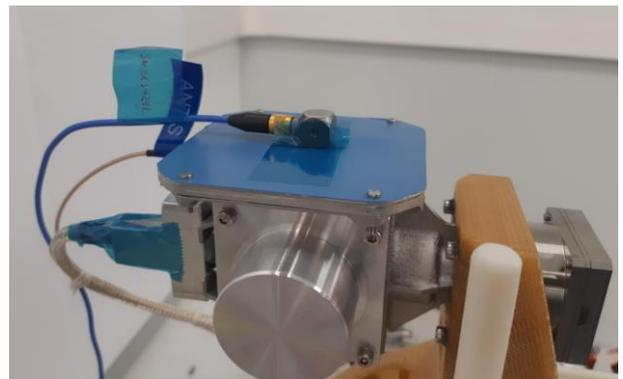
Figure 14. Accelerometer placed over camera box dummy.
