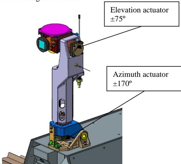
Figure 7. Deployment mechanism
