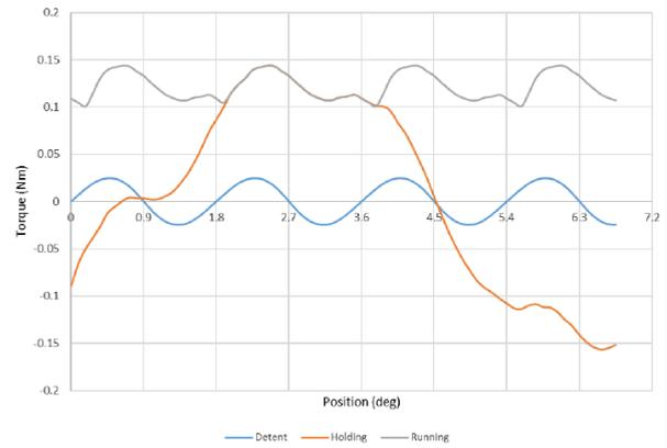
Figure 12. DTA4 torque results.
