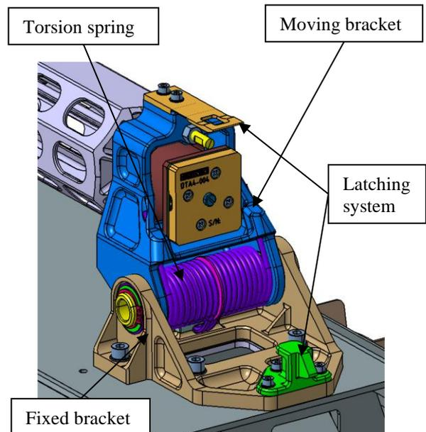
Figure 6. Deployment mechanism
