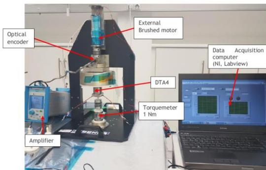
Figure 11. DTA4 holding torque test setup.
