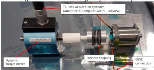
Figure 12. DTA4 running torque test setup.
