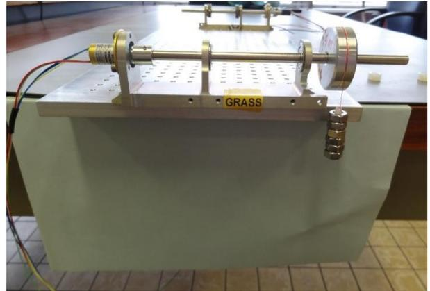
Figure 7. Torque measurement test setup with equivalent moment of inertia disc. Note that here the encapsulated Moflon slip ring was used for the test.
