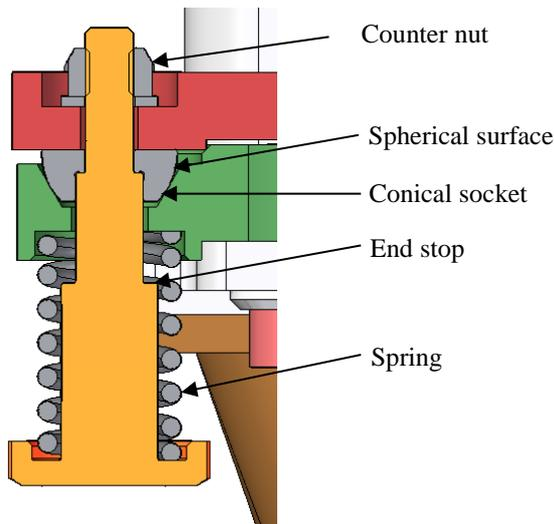
Figure 7. Receptacle's compliance mechanism
