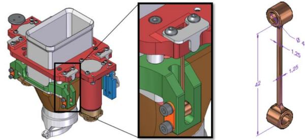
Figure 5. Initial concept of Plug compliance mechanism
