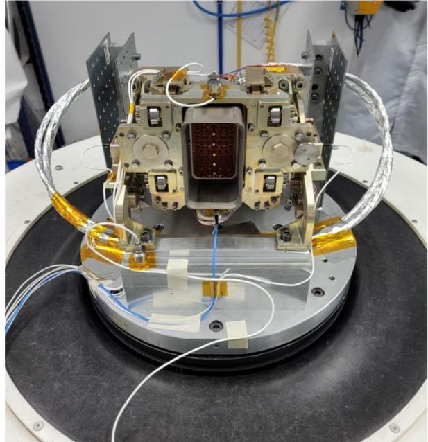
*Figure 10. RTU Plug mounted on the shaker*
