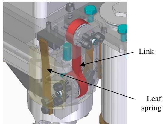
Figure 6. Final design of Plug's compliance mechanism
