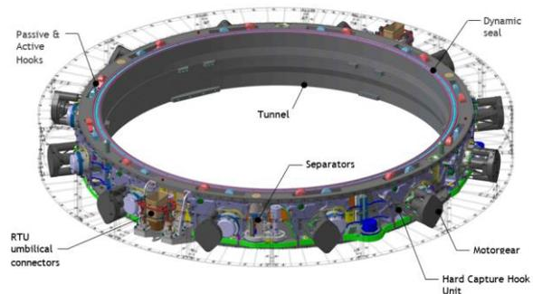
Figure 1. Hard Capture System main components (MMOD Cover outlined for clarity)
