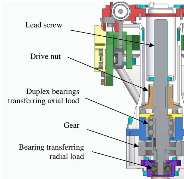
Figure 4. Cross section of lead screw – nut pair
