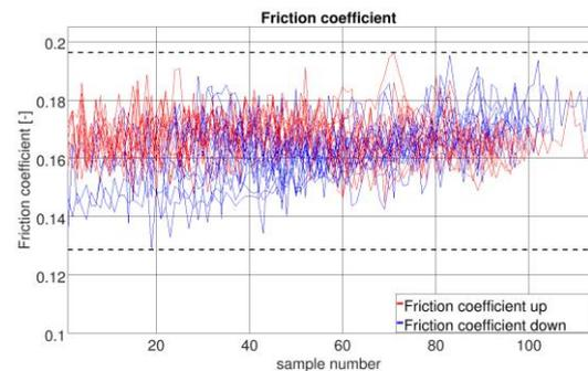
Figure 3. Friction coefficient of lead screw – driving nut pair in low temperature ( $-40^{\circ}\text{C}$ ), high vacuum ( $<0.1\text{ Pa}$ )
