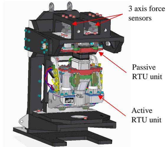
Figure 8. RTU functional test tool – general view
