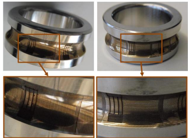
Figure 8. Oleophilic textures applied to B7004C-type bearing ring in perpendicular (left) and parallel (right) directions
