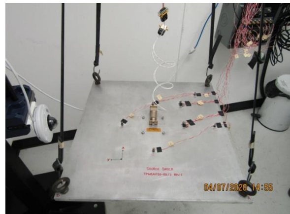
Figure 5 – Pin Puller Mounted on Shock Output Plate with Accelerometers
