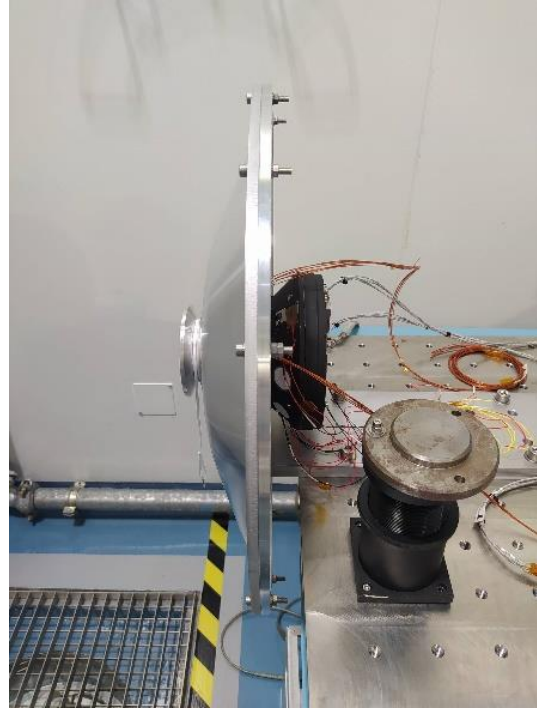
Figure 13. Encoder breadboard with flywheel
