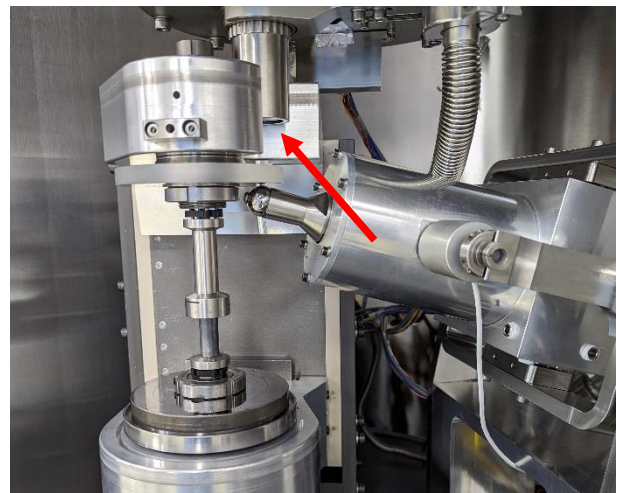
Figure 2: Image showing the optical disc measurement setup with the lens (arrowed) protruding into the cutaway.
