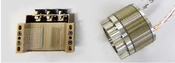
Figure 3. Picture of a traditional SRA (stator left side, rotor right side)
