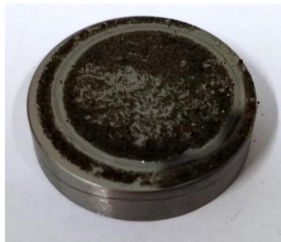
Figure 3. Surface of the sample with MoS 2 coating applied. After tribological test with JSC-1A powder.
