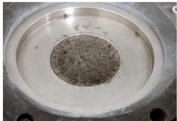
Figure 2. Surface of regolith-dusted MoS 2 -coated sample. Before testing.
