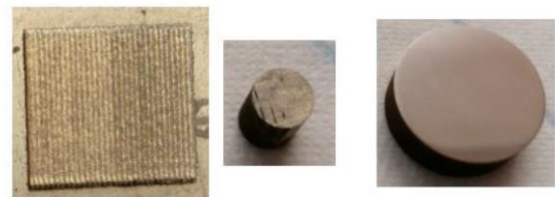
Figure 6: C1 (AMZ4) by LMD (as coated on steel, left), and machined pin (center) and disc (right).
