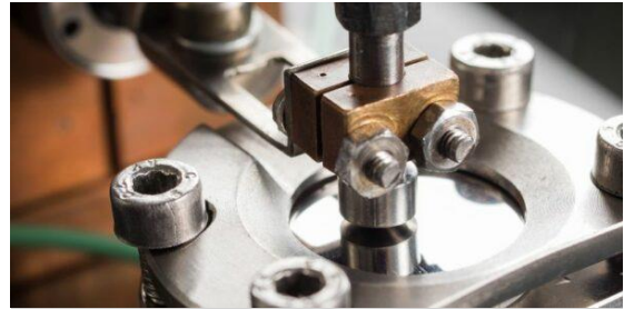
Figure 8: Fretting device: Detail showing the fixation of pin (upper rod) and disc (mounted directly on a force transducer).
