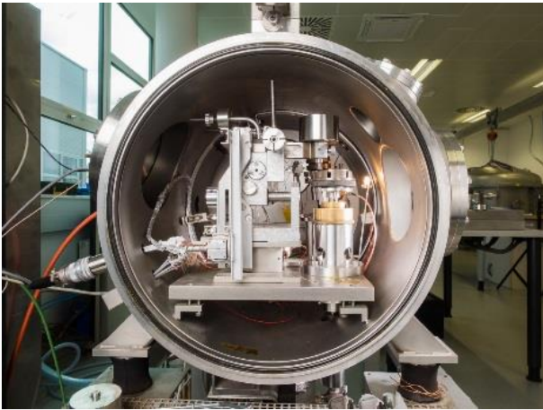
Figure 7: High Vacuum Tribometer (Inside view). Pin and disc holding, heating system not shown.
