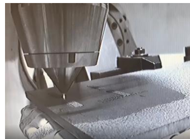
Figure 2: Nozzle deposition during patches realizations.
