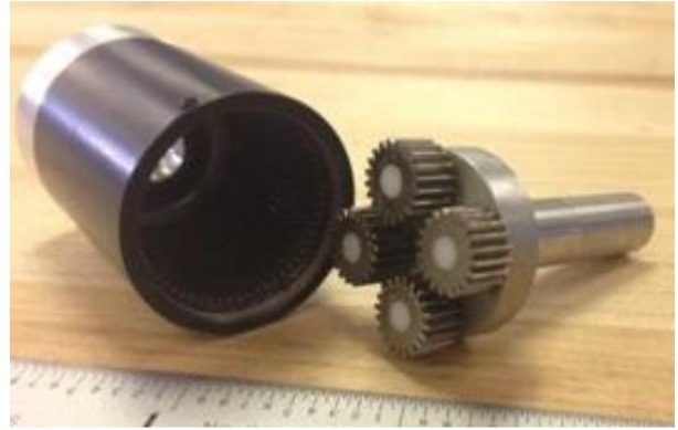
Figure 1: Components made of BMGs: Planetary Gear: Housing (left) Gear wheels on carrier (Right)
