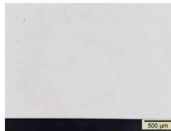
Figure 8: Microstructure after SCC-test of Cronidur X30 SCC at 75%RP0.2: No corrosion and no SCC-cracks.
