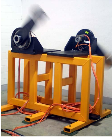
Figure 4: HD-gear endurance test rig
