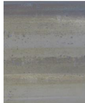
Figure 10: Raceway of outer WGB-ring of HD-Cron_1-2 after test: no wear identified
