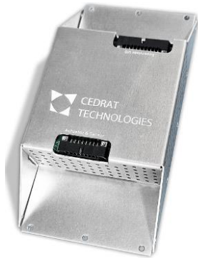
Figure 13. Rugged NewSpace version of the CCBu20 Drive Electronics
