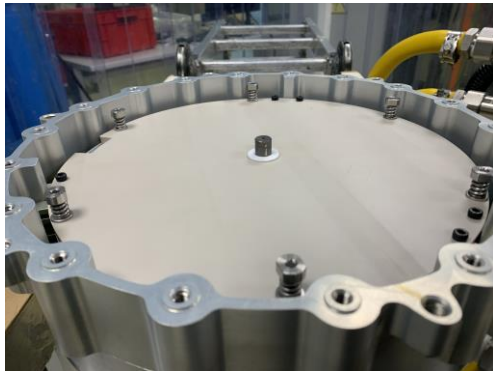
Figure 8. The vessel with holes for the enclosure, the preload springs, and the 4 TEG generators packaged.
