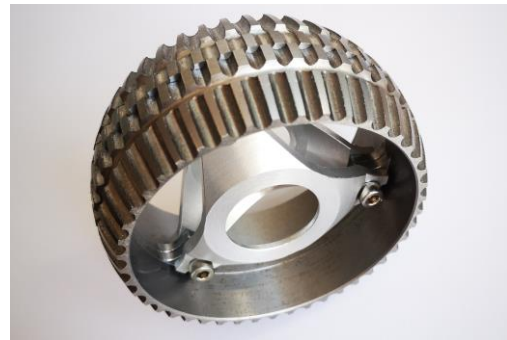
Figure 7: Prototype of the rotor of the M5GR4, manufactured on a conventional turning/milling machine
