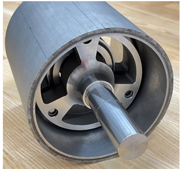
Figure 6. Subassembly of all the rotating components in the prototype cycloidal magnetic gear
