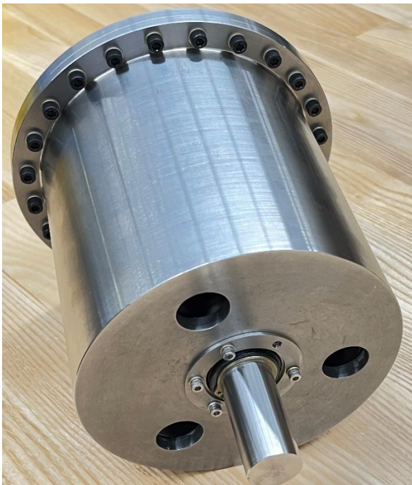
Figure 7. Assembled prototype cycloidal magnetic gear
