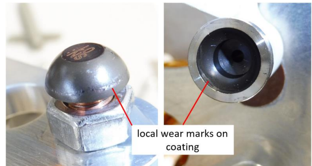
Figure 14 Wear marks on coating
