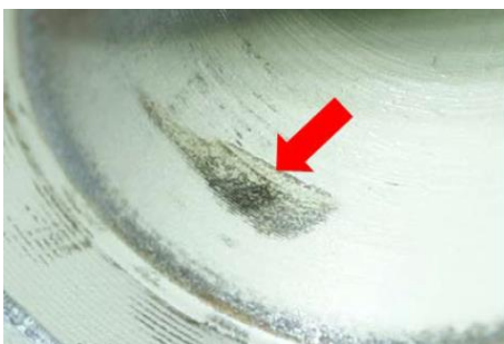
Figure 17. MoS2 transfer to the aluminium cup
